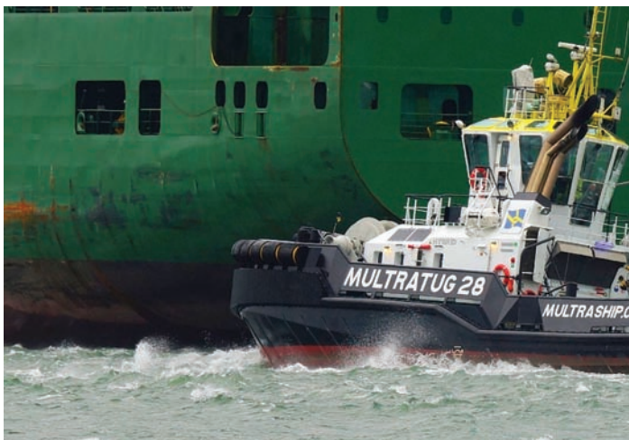
If ship uses the propeller, the tug will be in a dangerous position. Optimum pilot – tug master communication needed. Photo: Kees Torn, Tug Use in Port
