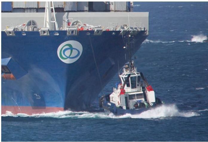
Risky situation near bow, tug preparing to pass towline. Photo: Kenneth Karsten, Tug Use in Port , 2021
