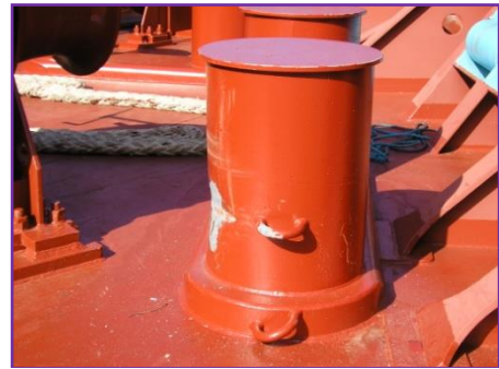
Courtesy: KOTUG, Rotterdam Top eye on bollard will damage the towline
